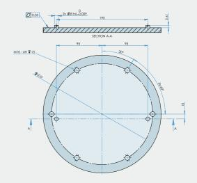
Recommended hole pattern for robot base
