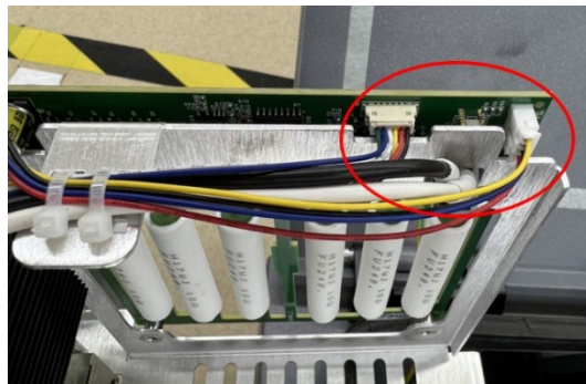
Figure 3-37 Reconnect the cable
