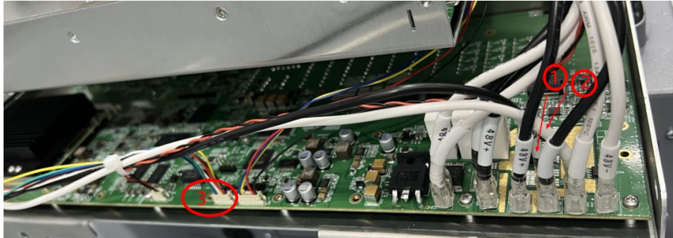
Figure 3-29 The position of cable from the brake pads to Safe IO
