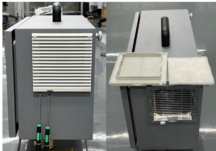
Figure 2-3 Controller filter disassembly and assembly
