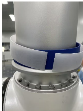
Figure 3-11 Remove the upper arm rubber ring and the supporting ring
